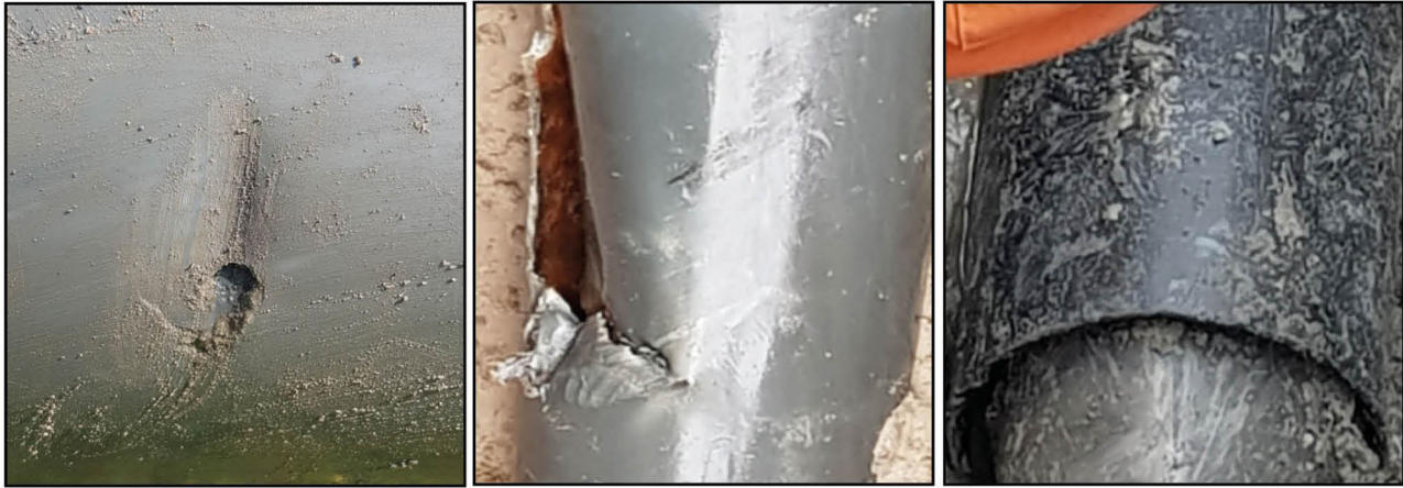
Figure 9. In-situ footage after excavation of pipes A-3 (left) and B-2 (middle) with break due to third party impact, and pipe B-3 (right) with crack due to poor installation quality.
